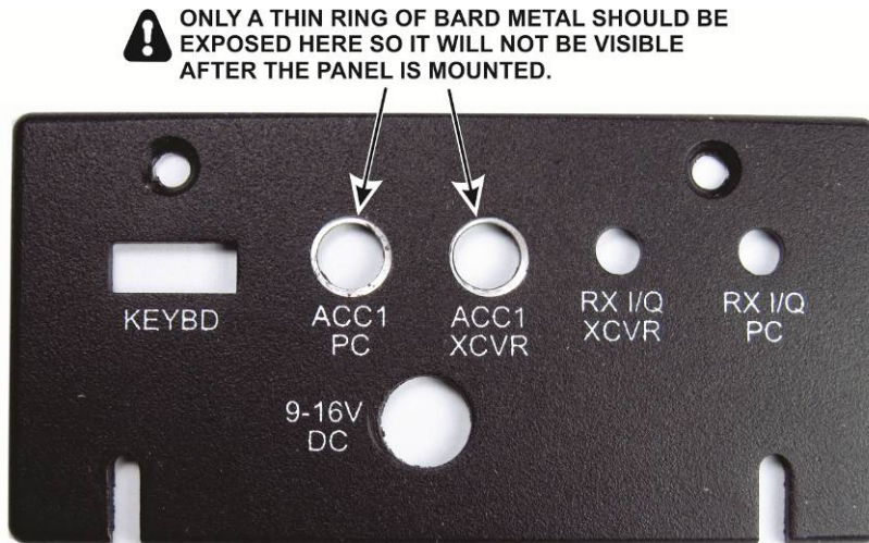
Figure 36. Checking the Grounding Surface on the ACC1 PC and XVCVR Connector Openings.
