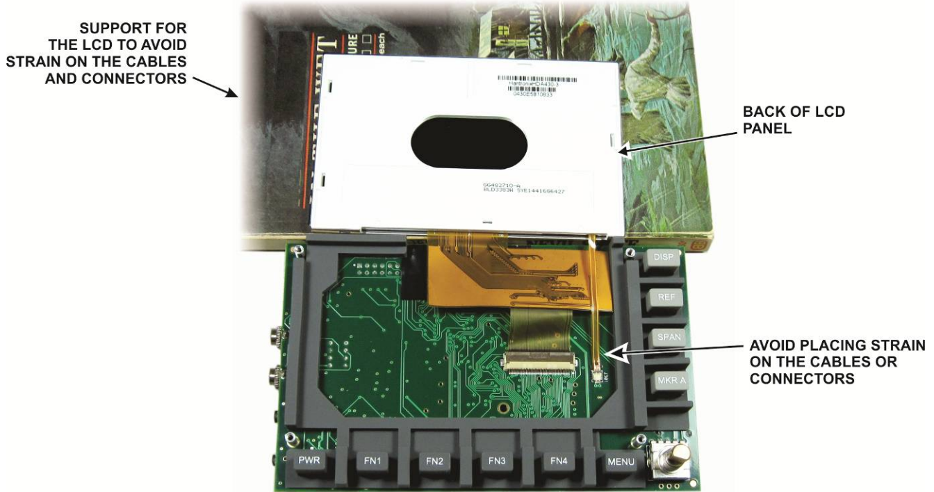
Figure 46. Removing LCD Panel from Rubber Key Matrix.
